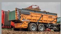
**Optimal loading space**: As the TC also functions as a folding rear tailgate, there is no additional rear overhang.
