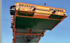
**Centering conveyor:** Damaged crops during the loading process are reduced to an absolute minimum thanks to the two optional centering conveyors.
