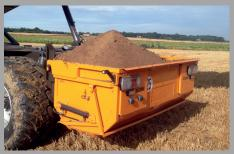
**No dirt on the road:** The soil is collected in the hydraulically operated soil-collector and can be unloaded evenly at a suitable location in the field.
