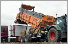
**Turbo output:** With a cleaning surface of +/- 5m², the TC can ensure both cleaning of the crop and loading lorries in short time. Less than 10 minutes are required to load a full lorry.
