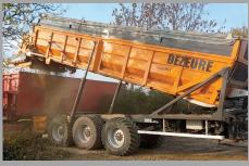
Unloading, anywhere at any time: The overload trailer unloads from the back, trailers can be loaded anywhere in the field.
