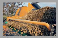
**Perfect cleaning:** The crop is nicely spread on the cleaning rollers thanks to the steady supply of crops by the discharge floor of the overload trailer.
